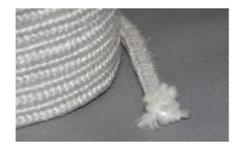
will withstand continuous exposure to temperatures of 1000°F / 520°C. This material resists most acids and alkalis and is unaffected by most bleaches and solvents. It is highly flexible and conformable.
